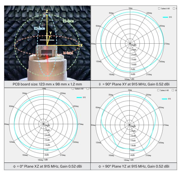
Note: Data tested with an evaluation board of 123 x 98 x 1.2 mm
